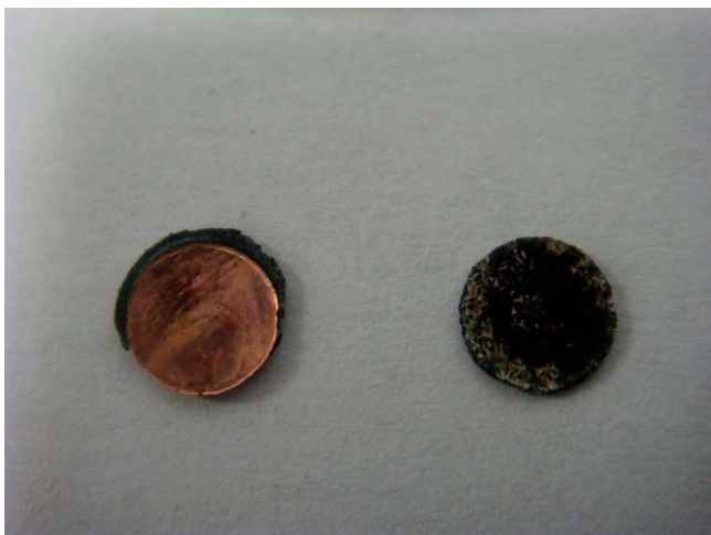
Fig. 2. The comparison of the anodes on Cu foil (left) and Ni foam (right) after cycling.
